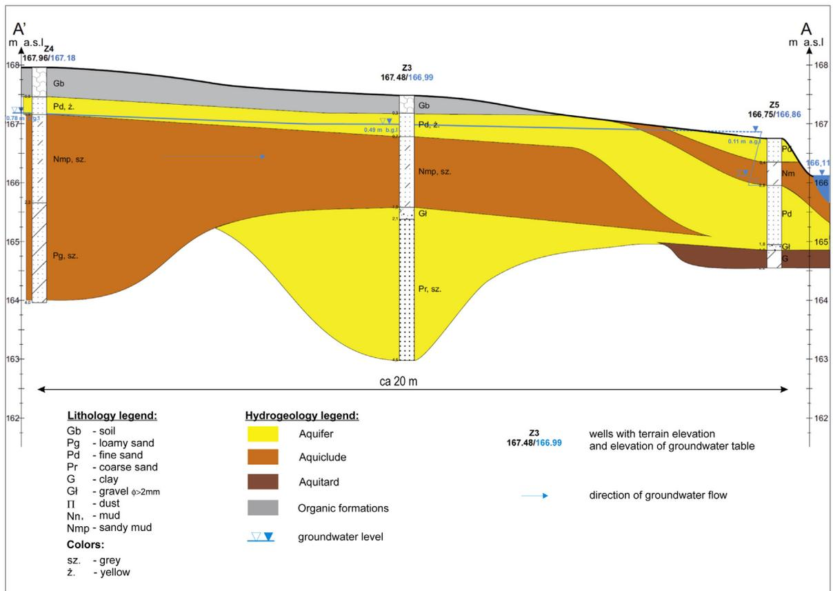
Fig. 2. Hydrogeological cross-section parallel to the stream valley.
