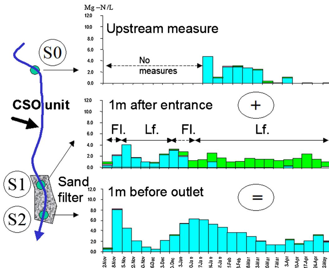
Fig. 14. Evolution for nitrate (blue bars) and ammonia (green bars) concentrations with time and space in a sand filter placed just downstream a CSO unit. S0, S1 and S2 are sampling sites from wells dug in the stream and sand substrates. Lf.: low flow period; Fl.: flood period. See experiment location in Fig. 13. (For interpretation of the references to color in this figure legend, the reader is referred to the web version of the article.)
