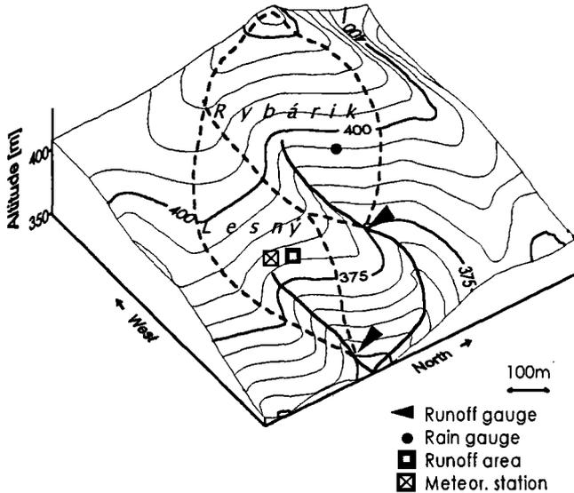
Fig. 1 Scheme of the experimental basins and equipment
