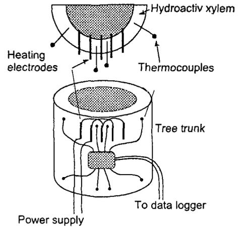
Fig. 2: Measuring device applied on tree trunks
