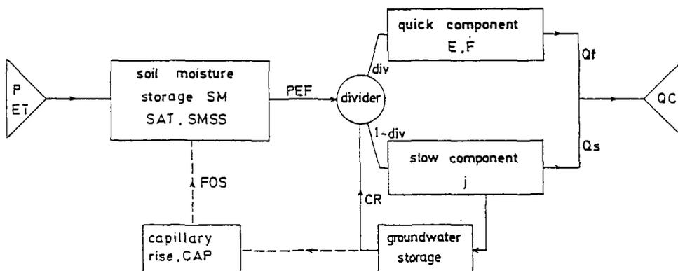
Figure 1: Flow diagram of the Wageningen mode:  $Q_f$  and  $Q_s$  are the computed fast and slow runoff components respectively and  $QC$  represents the total computed runoff.
