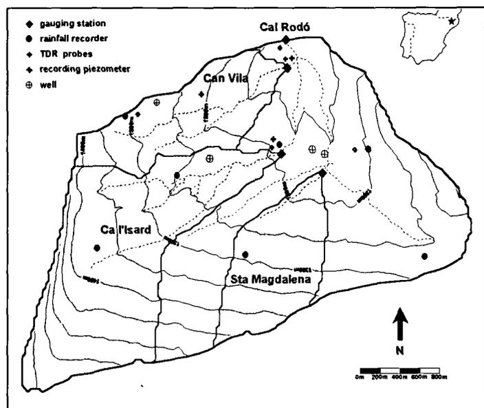
Figure 1: General arrangement of the measuring network.
