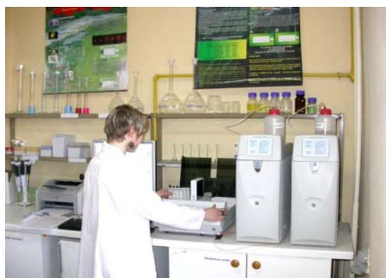
**Photo 2.** *Chromatograph for analyzing ions in water samples (European Regional Centre for Ecohydrology under the auspices of UNESCO, Lodz, Poland; photo: K. Izydorczyk).*
