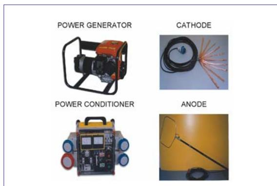
Figure 5. Electrofishing equipment (photo A. Bednarek).
